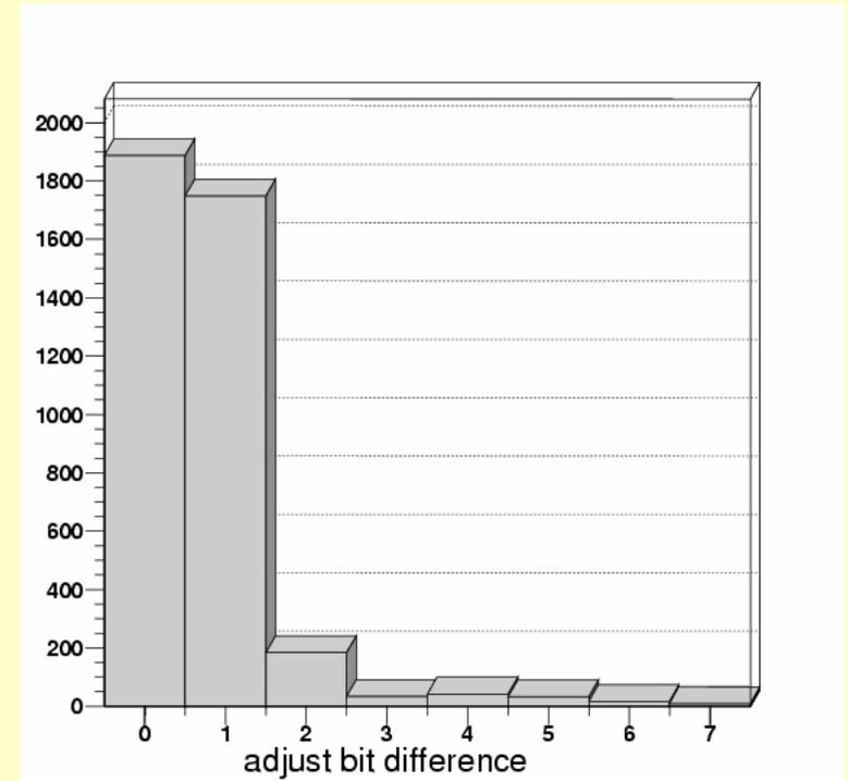
→ Main reason for different response of pixels is not the frontend: it is the spread of the response of pixel electronics that cannot be completely corrected
